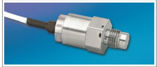
ETM-375 Series transducers are miniature, threaded instruments. The sensing sub-assembly is protected from mechanical damage by a solid screen which has been shown to have minimal influence on the frequency response of the sensor. Incorporation of a Kulite proprietary electronics module within the main body of this product allows
