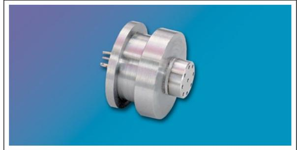
A **Low Cost** OEM component for downhole tools. Each transducer is supplied with a table of output sensitivity and bridge resistance values at various temperatures. When used with a fixed series resistor, these data provide the tool engineer with a low cost pressure sensor with a total error band of 0.25% (typical) over the entire operating temperature range of the tool.
