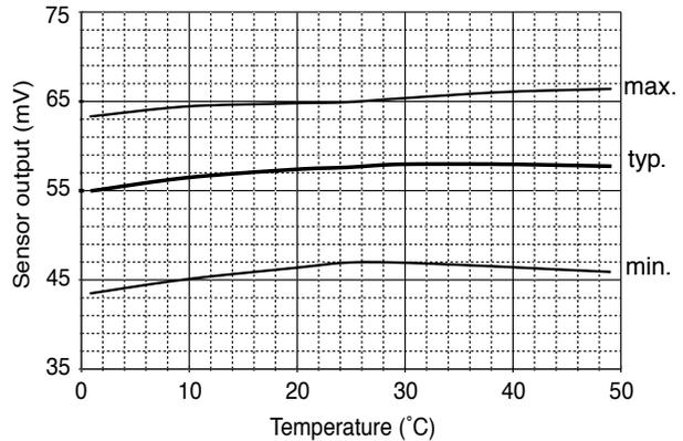
Fig. 8b - KE-50 temperature dependency of output voltage
