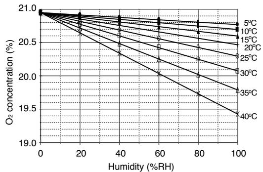
Fig. 7 - Effect of humidity on O<sub>2</sub> concentration
