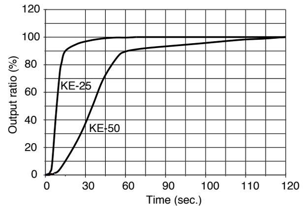
Fig. 4 - Response speed of KE sensors to oxygen
