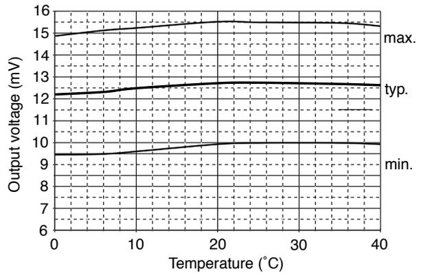
Fig. 8a - KE-25 temperature dependency of output voltage
