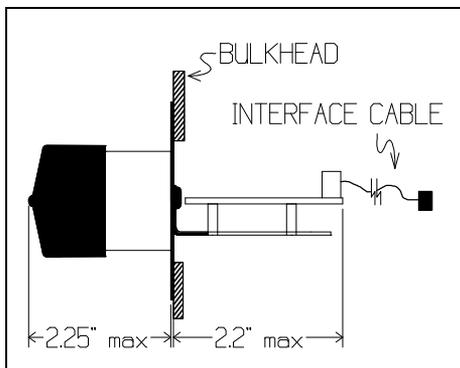
**Figure 1:** Typical Bulkhead Style Detector Mounting
