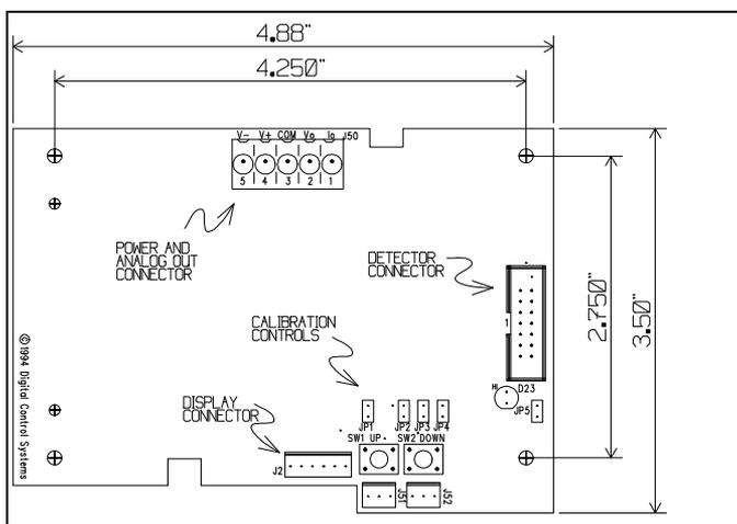
**Figure 3: Control Board Layout**
