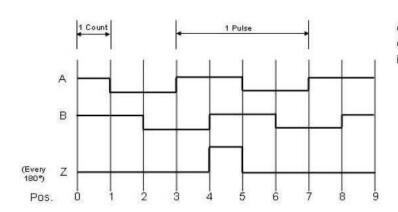
Channel A leads when Channel B shaft is rotated in Clockwise direction.
