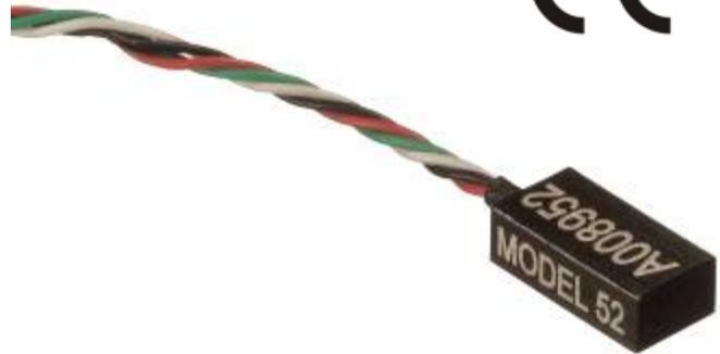
**The Model 52 Accelerometer** is based on an advanced piezoresistive MEMS sensing element which offers exceptional dynamic range and stability. This unit features a full bridge output configuration with an operating temperature range from -40 to +121°C. A slight amount of internal gas damping provides outstanding shock survivability and a flat amplitude/phase response up to 7kHz.
