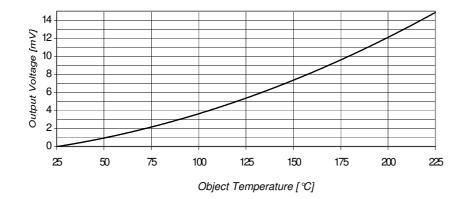
Conditions: Distance Thermopile/Black Body 5 cm, emissivity= 1, surrounding temperature 25  $^{\circ}$ C
