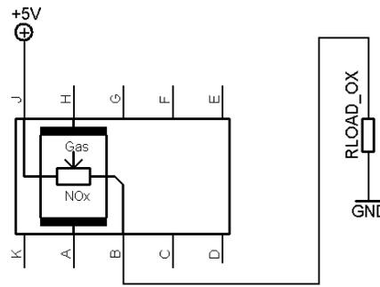
MiCS-2714 with measurement circuit (top view)
