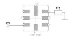
MiCS-5526 with recommended supply circuit (top view)
