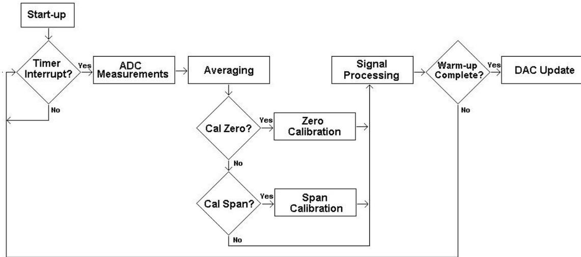
Figure 1 – Flow Diagram of Software Layout
