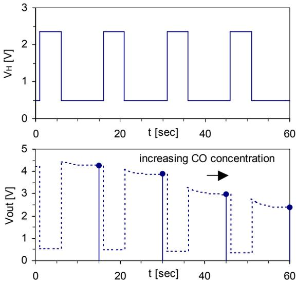
**V<sub>H</sub> and V<sub>out</sub> as a function of time with CO**
