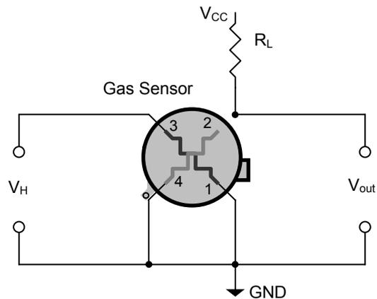
**Measurement circuit for CO detection**
