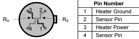
**Equivalent circuit (top view) of MiCS-5525**
