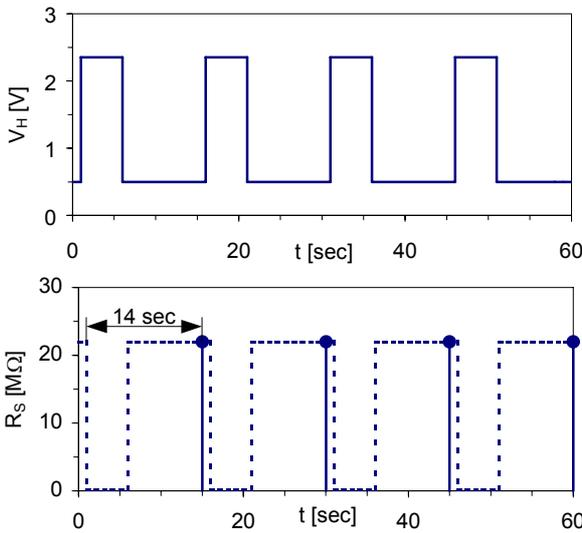
**V<sub>H</sub> and R<sub>S</sub> as a function of time without CO**
