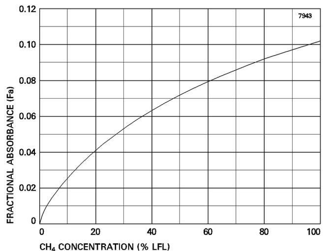
**Typical Sensitivity to Methane (100% LFL = 5% vol.) (IR32BC, IR42BC)**
