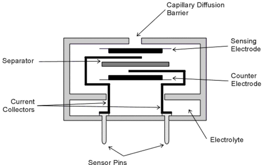
The electrodes need to be kept apart and wetted with an acid electrolyte to allow an ionic current to pass between them. This is done using discs of inert absorbent material or separators. These can be made from materials such as glass fibre.
