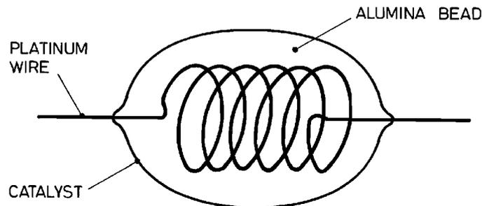
The design has been modified to reduce the amount of power used by the sensor and to make the sensor more resistant to poisoning and mechanical shock. e2v, when known as EEV, was in the forefront of these developments and the current range of pellistors incorporates the design improvements.
