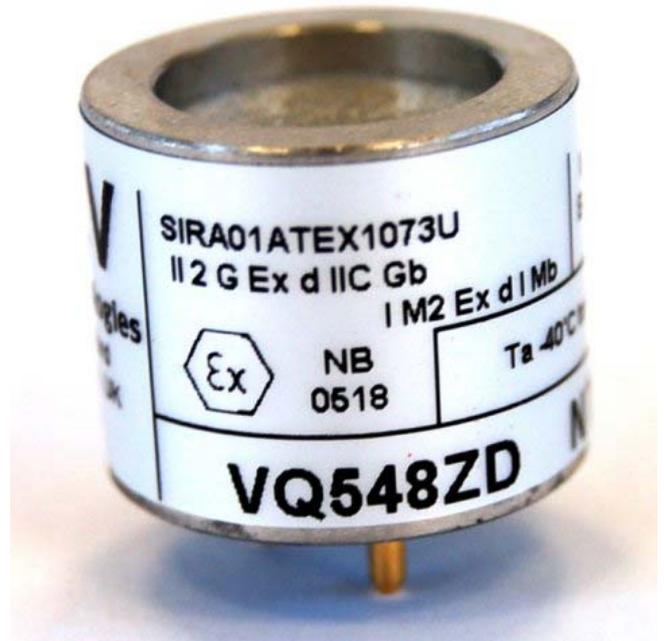
For the VQ548ZD/W, a carefully matched set of detector, compensator and resistor are encapsulated in a cylindrical stainless steel housing with an integral stainless steel sinter at one end to permit the entry of the atmosphere. Electrical connections are made to three pins at the other end of the body.
