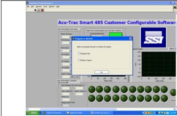
The system setup dialog asks if you would like to program the Smart 485 level transducer or monitor the output.
