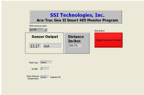
The program will refresh the data on the screen based on the update rate that is programmed into the part.
