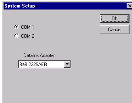
The system setup dialog provides the means to change the communications port on your PC for the RS-485 to USB adapter being used.
