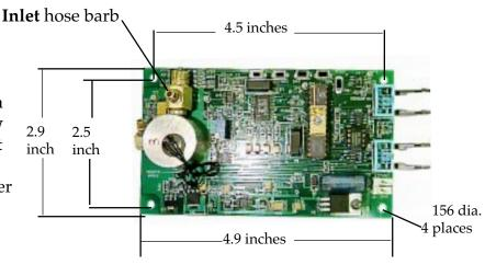
See **Application Note A67** for gas conditioning requirements and information about gas sample pumps and filters. A **hydrophobic filter** (**App Note A79**) in front of the **inlet** hose barb is required to prevent particles & droplets from entering the gas cell. Try to minmize the outflow resistance to minimize the back pressure inside the gas cell.
