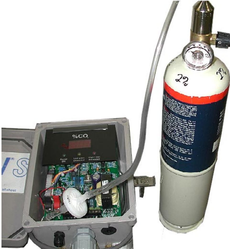
See the **specification sheet** for the specific full scale **Model 2166** you are calibrating and find the response scale chart that shows both the 0 to 5 volt and 4-20 mA outputs as a function of gas concentration. As an example, a 1% CO<sub>2</sub> full scale unit should have a 2.50 volt output or 12.0 mA output for certified 0.5% CO<sub>2</sub> span gas.
