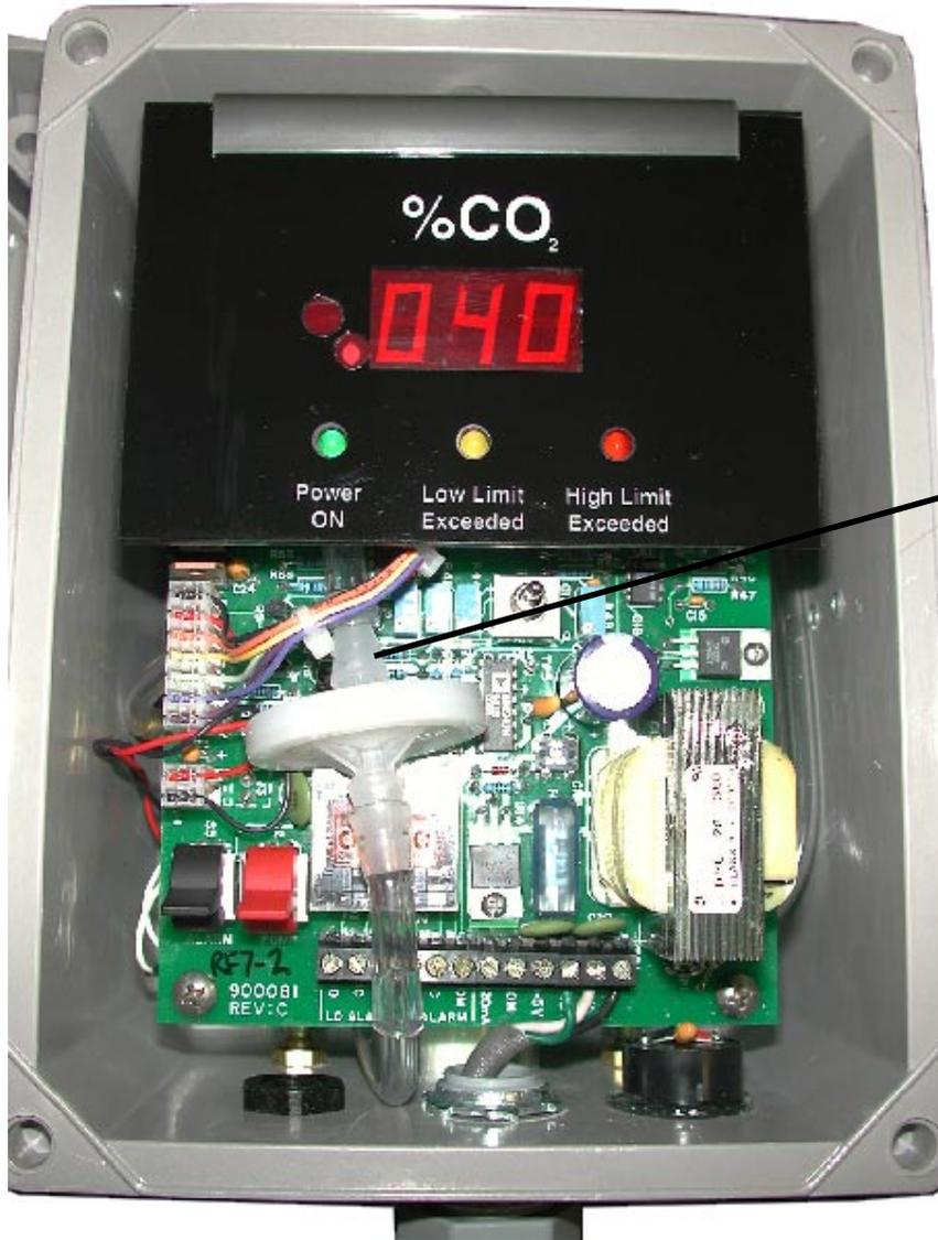
**INLET** side of Hydrophobic filter. See **Application Note A24** for complete gas calibration instructions.
