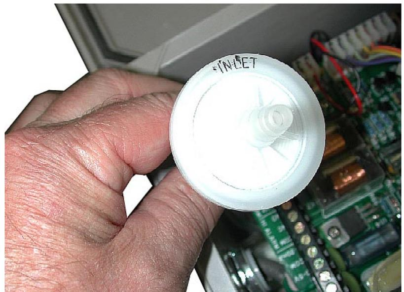
Using the INLET side of the hydrophobic filter to conserve calibration gas by using a lower flow rate.
