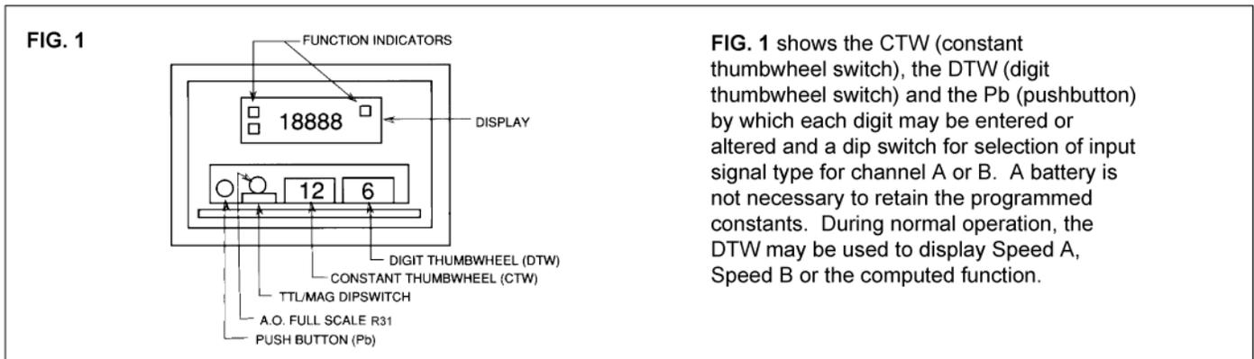
FIG. 1 shows the CTW (constant thumbwheel switch), the DTW (digit thumbwheel switch) and the Pb (pushbutton) by which each digit may be entered or altered and a dip switch for selection of input signal type for channel A or B. A battery is not necessary to retain the programmed constants. During normal operation, the DTW may be used to display Speed A, Speed B or the computed function.
