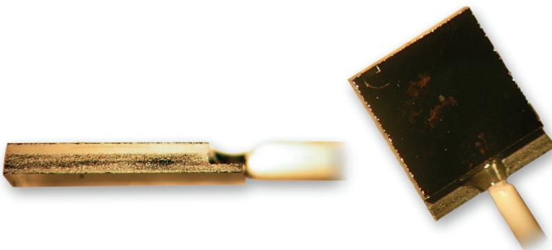
The FOP-MSL is a fiber optic pressure sensor designed for general industrial applications. Designed to fit where standard sensors cannot, FISO'S side-looking fiber optic pressure sensor features complete immunity to EMI and RFI and offers built-in safety for hazardous environments.
