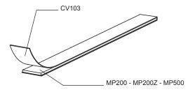
Width 10 mm – Thickness 0.3 mm. To be applied on magnetic tapes MP200 – MP200Z – MP500.
