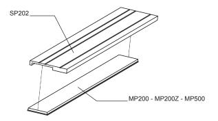
To be fixed on the machine to support the magnetic band.
