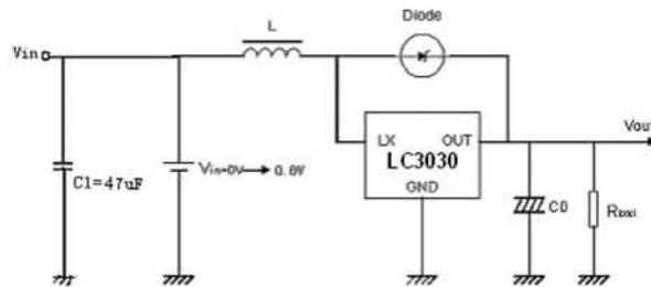
Hold-on voltage test circuit
