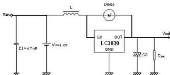
Start-up voltage test circuit
