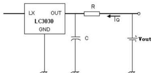
Oscillator frequency and duty cycle test circuit
