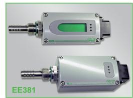
$a_{w} = 0$  corresponds to water-free oil, while  $a_{w} = 1$  indicates saturated oil.  $a_{w}$  measurement with the EE381 transmitter is based on the outstanding long term stability and resistance to pollution of the E+E capacitive sensor elements series HC.
