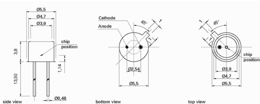
Selection code "18S" → TO18 Ni plated short housing, 5.6 mm diameter, 3.8 mm height two gold plated pins (Anode grounded and Cathode isolated). Not available with filters.
