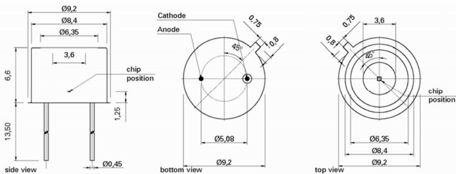
Selection Code "5" (photodiodes with filters) → TO5 Ni plated housing, 9.2 mm diameter, 6.6 mm height, two gold plated pins (Anode grounded and Cathode isolated).
