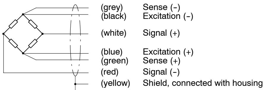
Electrical and magnetic fields often are the cause for the introduction of disturbing voltages into the measuring circuit.
