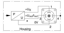
HS6P plug EMC up to 3V/m\*\*\* (corresponds to MIL plug PT02E-10-6P)
