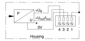
HAN7D/8U plug (8 pin, manufacturer Harting company) EMC up to 3V/m\*\*\*
