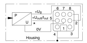
DIN 43 650 plug EMC up to (DIN IEC 803-2\*\*)
