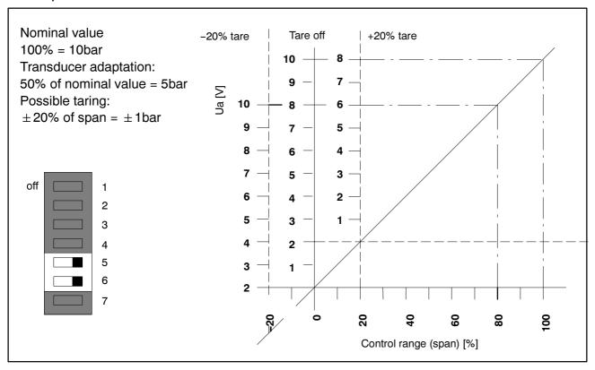
With the P19, the initial point can be shifted up to  $\pm 20\%$  of the output span. For this, activate switches S5 and S6 (on) and use potentiometer "Z" (ZERO) to suppress the output signal resulting from the initial pressure except for a residual signal of approx. +30mV (or e.g. 0.06mA at output 0...20mA). Shifting the switches 5 and 6 to the "off" position deactivates the tare function.
