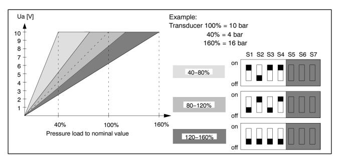
The zero point must be adjusted prior to span adjustment. Taring (switches 5, 6) and 7 must be set to "off".
