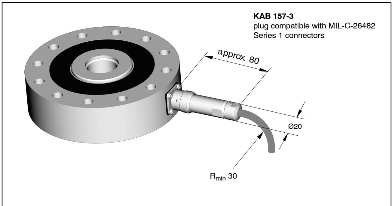
**Fig. 8.1:** Space for the bayonet locking connector
