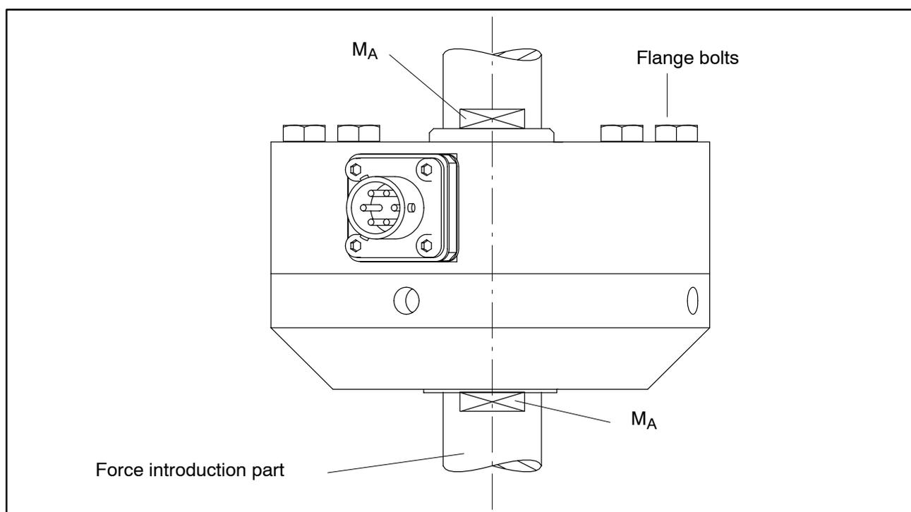
**Fig.4.2:** Installation with an adapter for tensile/compressive loading
