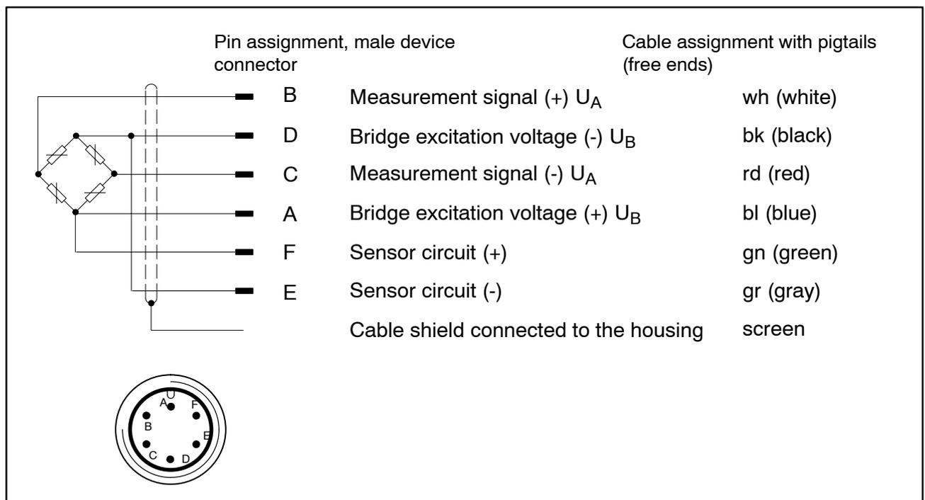
**Fig.5.1:** Cable assignment KAB 157-3 and KAB 158-3
