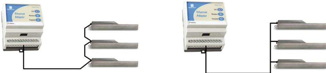
Figure 31: Correct RS485 cable network
