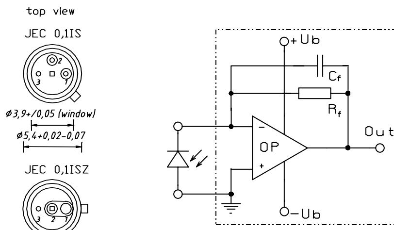
The application example shows a typical circuit..  $R_f$  is responsible for the gain of the circuit.  $C_f$  compensates the reverse junction capacitance of the photodiode and input capacitance of the OPV. The exact value of  $C_f$  depends on  $R_f$ , used OPV and capacitance of the circuit. A typical value is 1 pF.
