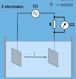
AC excitation is recommended to reduce degradation of the electrode and electrolyte
