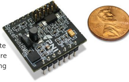
The SCOUT is designed for use in highly dynamic conditions such as high-speed gaming, remote controllers where accuracy is demanded, robotics, and limb and body tracking virtual reality...essentially any applications that require stable and repeatable tracking of physical movement.
