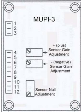
*NOTE: By increasing the gain, electrical 'noise' will also increase, and other performance parameters may be affected. It is suggested that all performance specifications be subsequently verified once the gain has been modified. Regardless, it is not recommended to increase the gain above a factor of X3!*
