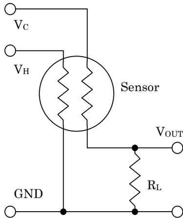
Pins 1 and 3 on the TO-39 header are attached to the heater. Apply  $V_H$  across these pins.
