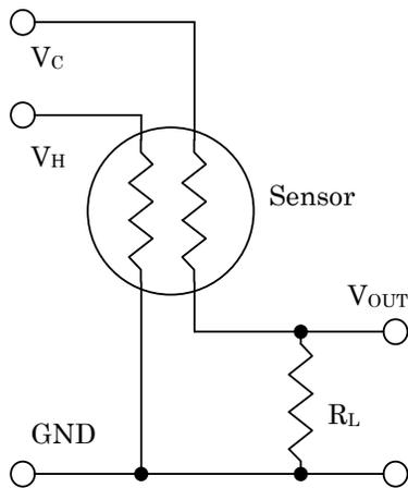
Pins 1 and 3 on the TO-39 header are attached to the heater. Apply  $V_H$  across these pins.
